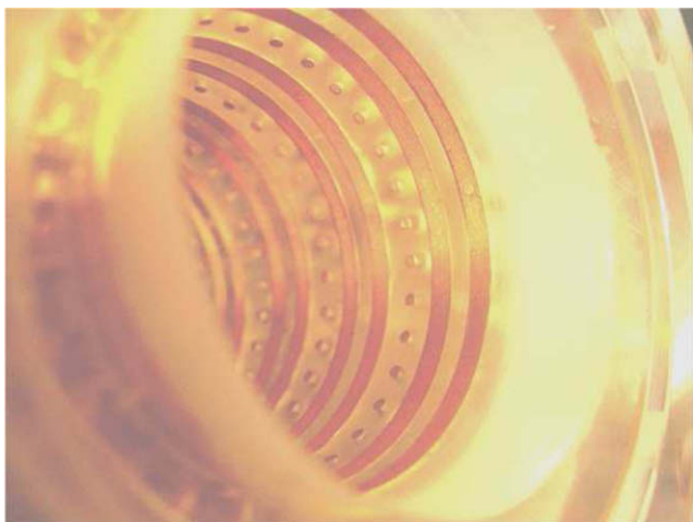
Fig. 2. Picture of the film thickness sensor. The conductance is measured between a ring-electrode and island-electrode flush with the wall.
